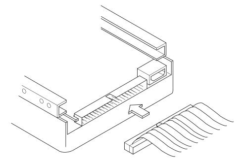
Step 3. To plug in additional internal SCSI devices, use an internal SCSI ribbon cable with the required number of 68-pin connectors attached along its length as shown in Figure 2.6.
